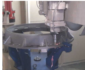
Bolt hole burr grinding
