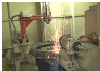
Due to a small tool NO.1, core print burr grinding
